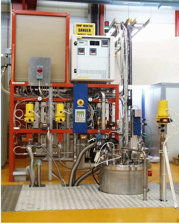
(a) Test station with down cryostat and probe holder. The magnet is below the platform.
