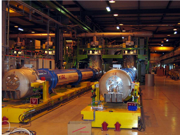
Figure 2.19: Test stand for cold measurement with two dipole magnets (blue).
