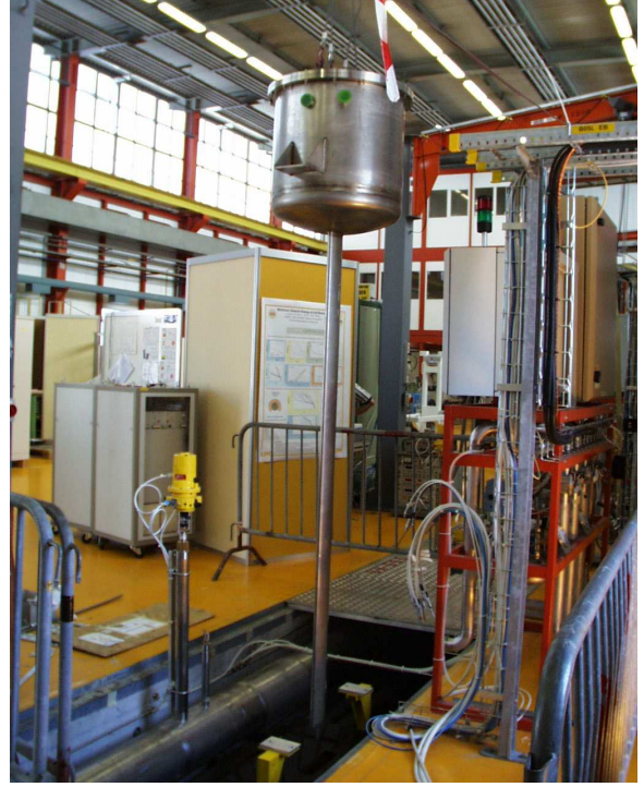
(b) The long metal shaft contains the strands to be measured. The big tank is filled with super fluid helium in order to provide the measurement temperature of 1.9 K for suitable time span.
