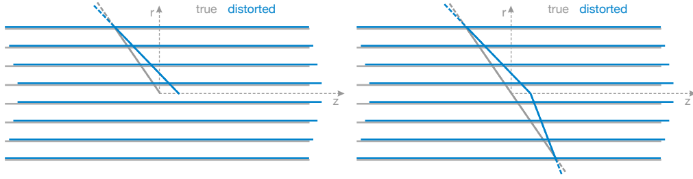
Figure 3.2: Diagram demonstrating distortions of the tracker geometry that may not affect the consistency of a reconstructed collision track with the measured hits (left), but introduce a kink when reconstructing the two halves of a cosmic ray muon track (right), leading to an inconsistency. This illustrates the telescope effect from Table 3.1.
