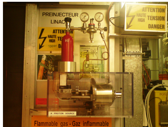
Figure 4.2: LHC protons originate from a small hydrogen bottle, pictured here with the duoplasmatron. [141]
