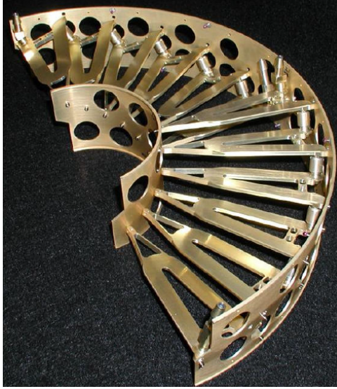
Figure 2.5: Phase-0 FPIX half-cylinder support structure. The FPIX half-disk cooling channels are mounted in the outer half-ring structure, and the panels are mounted on both sides of the cooling channels [40].
