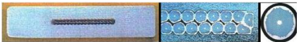
Figure 1.3. Cross-sections of the conductor used in ATLAS barrel toroid. On the left is the full conductor, sized 12×57 mm 2 , in the middle a detail of the cable and the bonding between Al and Cu, and on the right the Nb-Ti/Cu strand of 1.33 mm diameter [12].
