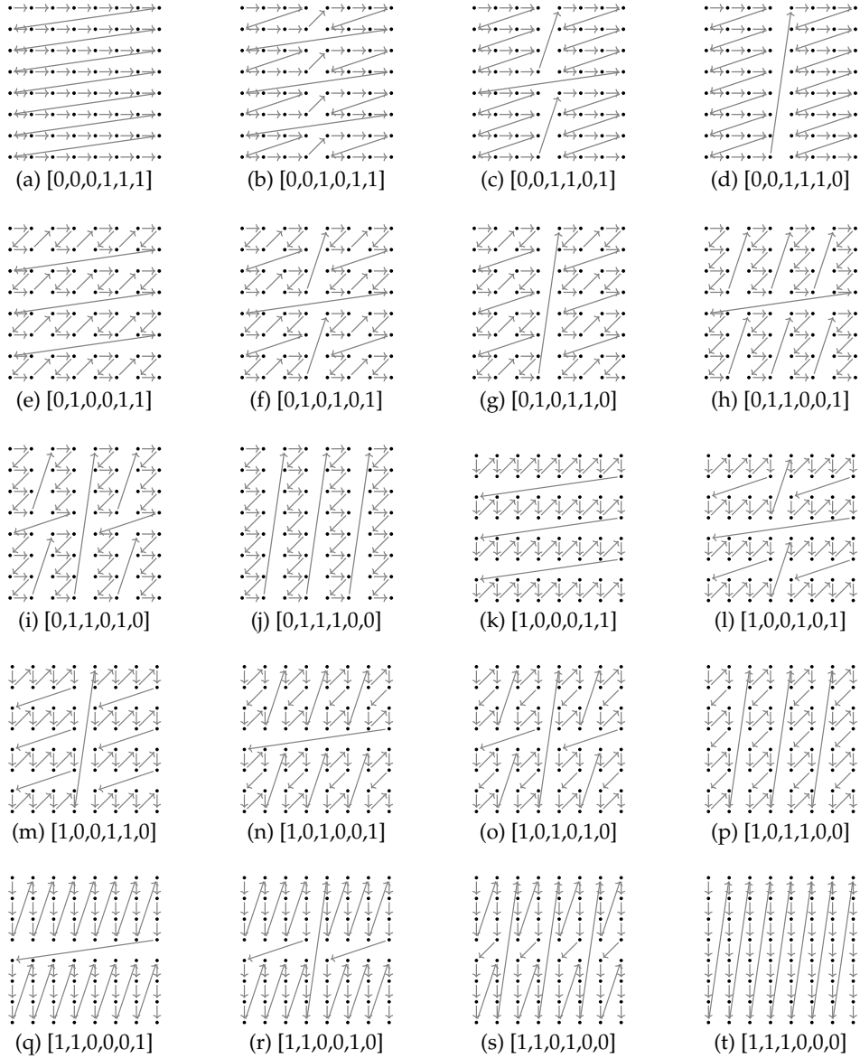
Figure 6.2: All 20 layouts for 8 \times 8 arrays generated by the family of indexing schemes described in Section 6.3. Note that Figure 6.2a corresponds to a row-major layout, while Figure 6.2t corresponds to a column-major layout.
