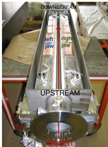
Figure 7: an LHC collimator [14]
