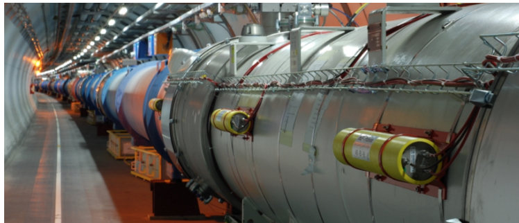
Figure 12: Beam Loss Monitor attached on a focusing quadrupole [14]
