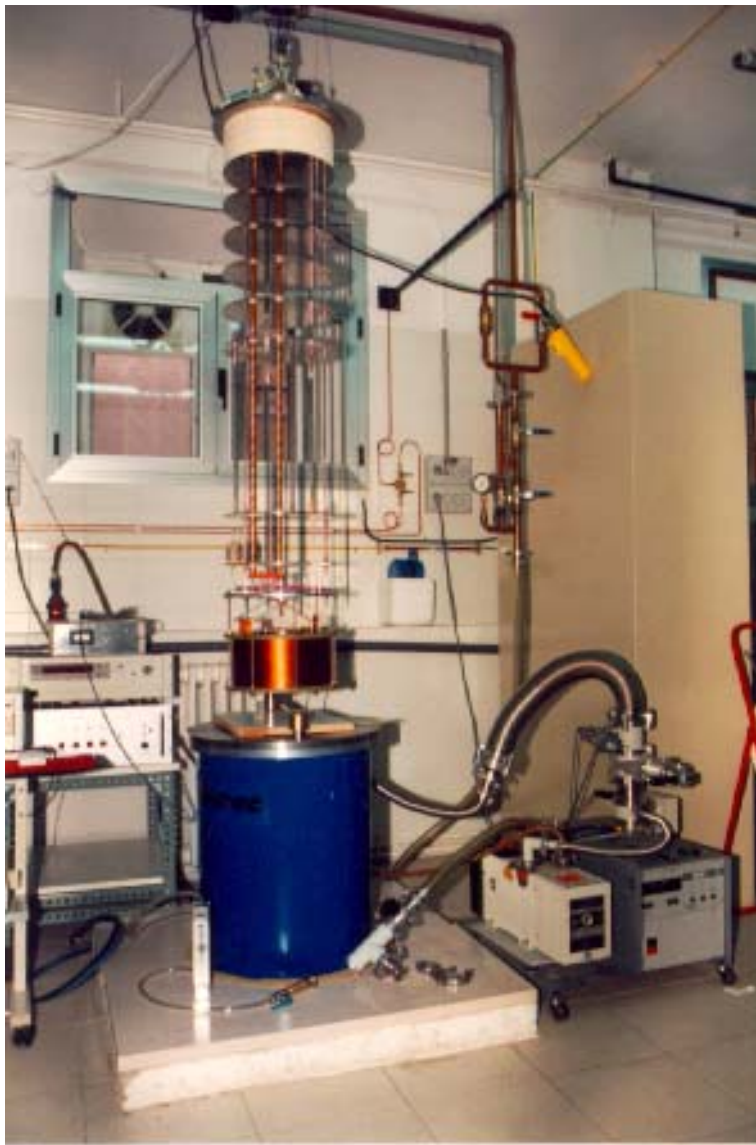
Figure 4.2: View of the cryostat, support and coil of the 25kJ SMES designed and built in Spain
