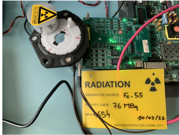
Figure 7: Laboratory setup for charge calibration with Fe-55, a radioactive source of photons with the fixed energy of 5.9keV
