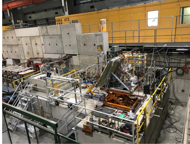
Figure 5.17: The H8 beam line of SPS at Prevessin North area of CERN which the Micromegas testbeam experimental setup is installed.
