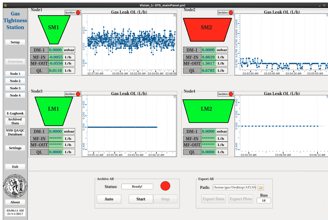
Figure 4.32: Check the sensors and MM QP of each node with 4-Node Mode in the FRL method.
