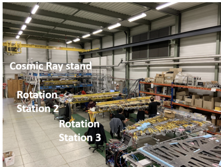
Figure 2.12: The cosmic ray stand along with the rotation stations at BB5 during the integration of the Micromegas electronics and wedge preparation.
