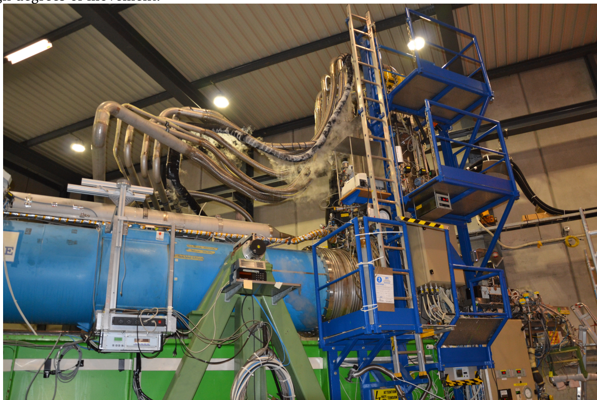
Figure 5-6 Cryo flexibles condensing atmospheric oxygen and water during a Quench.
