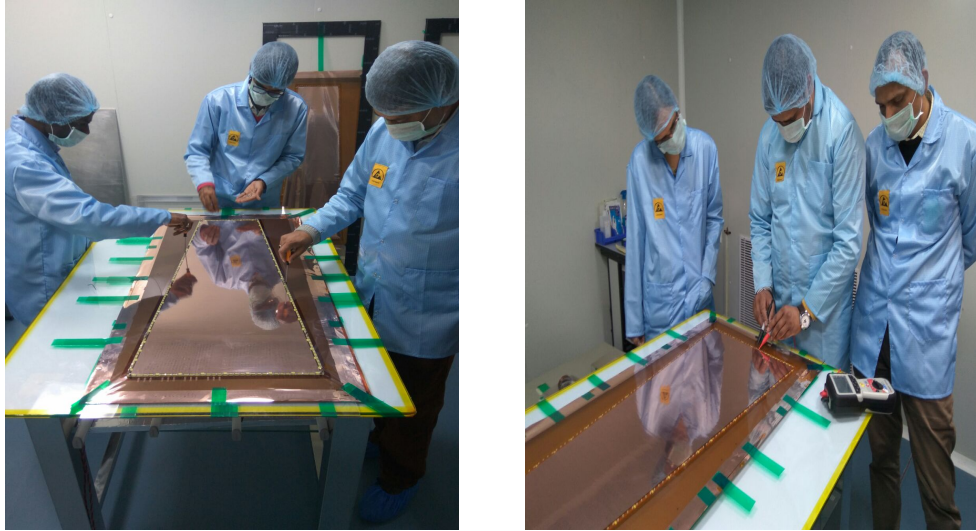
Figure 2.21: Placing the metallic screws in the spacers (Left). Testing the GEM foils using the Megger (Right).
