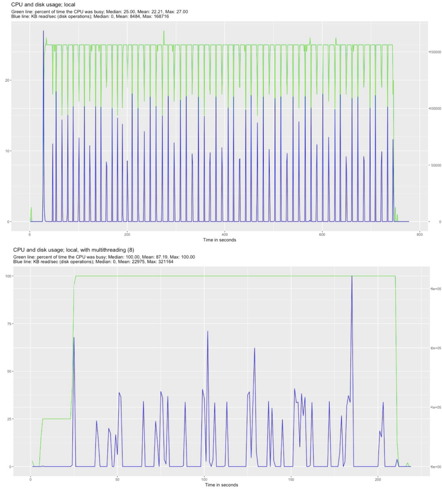
Figure 11: CPU usage and kilobytes read from SSD in time of application execution
