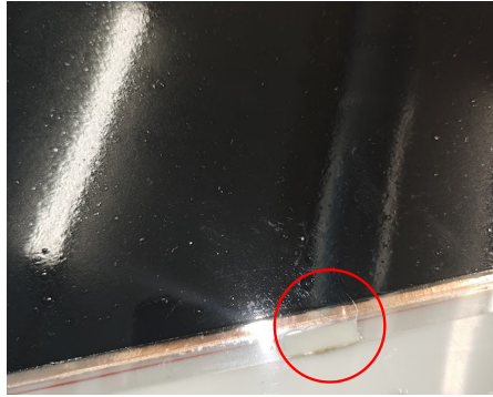
Figure 16: Detector 1: fracture on the bottom glass near a spacer (highlighted in red).
