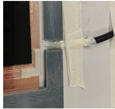
(c) Gas pipe glued into the port (close-up).
