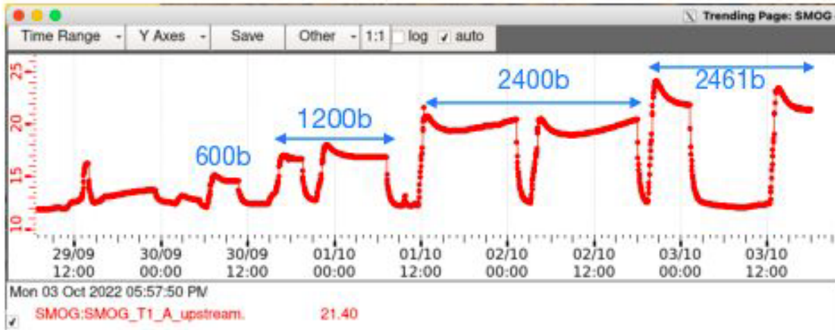
Figure I.4.11: Trend of the temperature readings from one of the thermocouples over four days during the 2022 run; the period of time corresponding to beam injection are reported, with the intensity indicated. A clear correlation between the temperature rising and fall and the presence of the beam can be observed.
