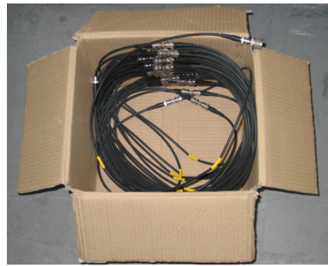
(b) LHC in the box: these BNC cables give an idea how a 700m long section of beam-pipe will behave at high frequencies.
