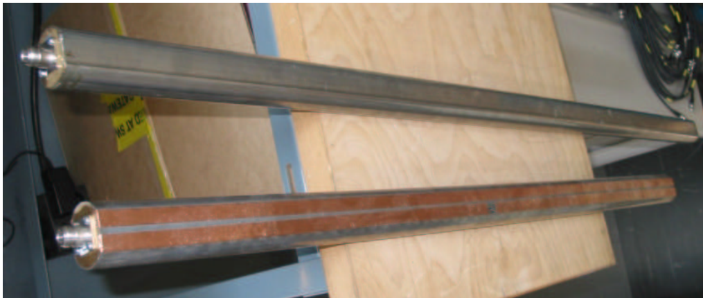
Figure C.5: The two beam-pipe resonators. The slotted one was just being prepared for the radiation measurements by covering the holes with copper bands
