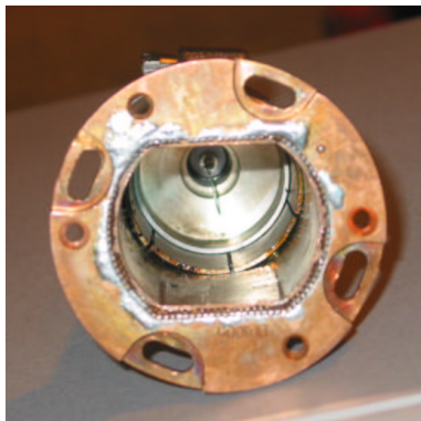
(a) A look inside reveals a TE type mode launcher.
