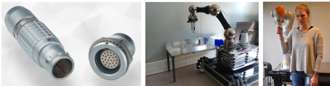
Figure 5.43: Picture of the Lemo B-type standard self-latching multipole connectors, with alignment key, used for the test (left), the connection task being performed by CERNbot in single arm configuration (center) and an operator at the master station (right).
