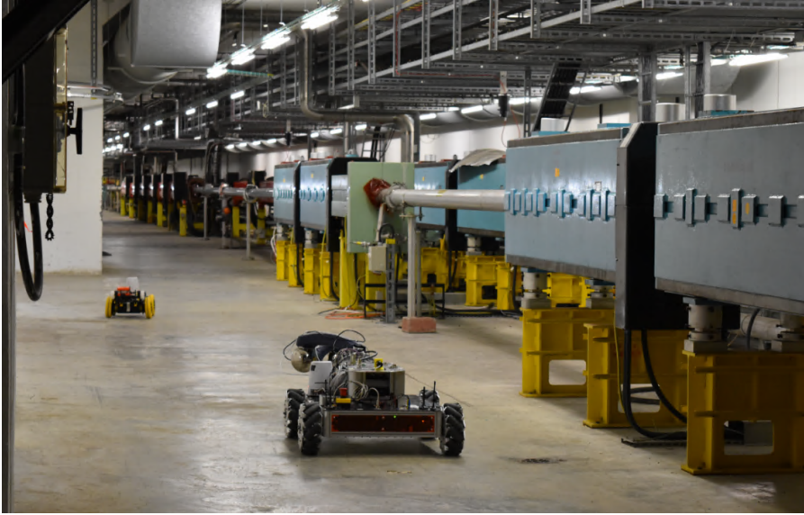
Figure 6.25: CERNBot v1.0 and EXTRM in North Area beamline
