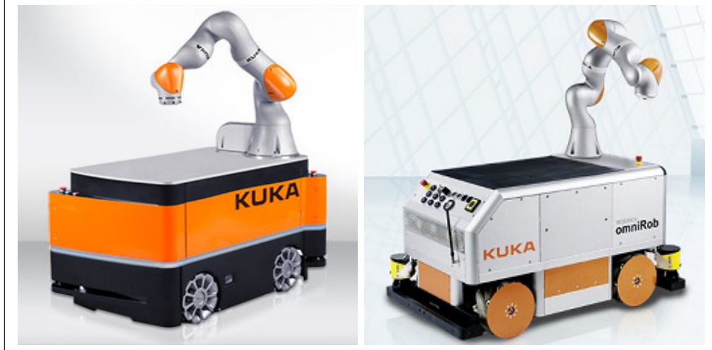
Figure 1.1: Kuka Omnirob mobile manipulator (adapted from [55])
