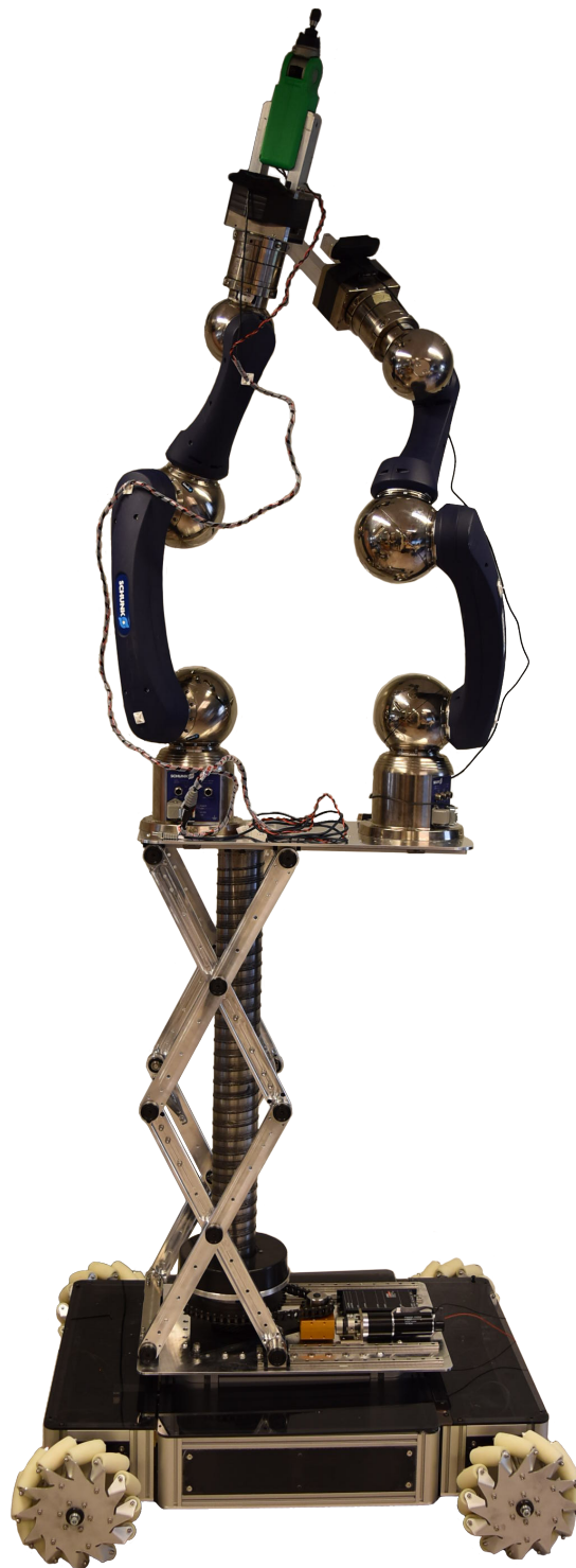
Figure A.19: The CERNBot2 with the stage up carrying dual robotic arms.
