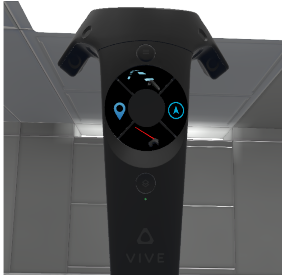
Figure 5.28: Four functions displayed in HTC VIVE controller. Teleport(Up), Map(Left), Navigation(Right) and laser(Down).
