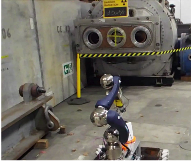
Figure 6.3: CERNBot 1.0 while approaching the radioactive object discovered in the area
