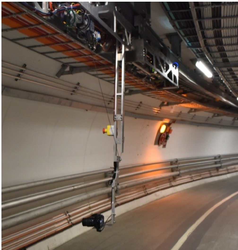
Figure F.5: Camera in the proposed orientation, such that it is facing the wall, capturing images containing a 'plain' background with wall cracks and other defects as foreground.
