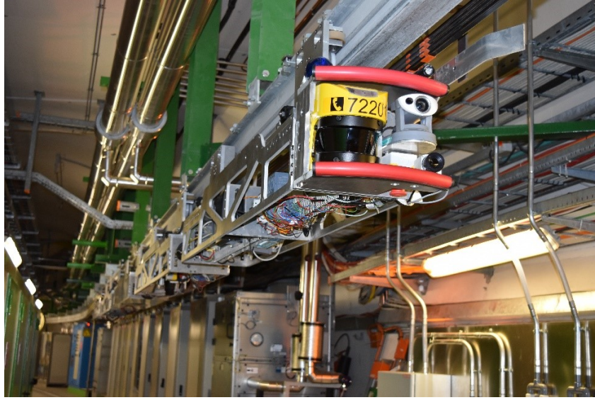
Figure A.1: The Intelligent Train Inspection Monorail (I-TIM)
