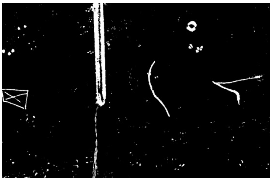
Figure F.20: Neighbourhood image differencing with a low threshold value as used in the algorithm.
