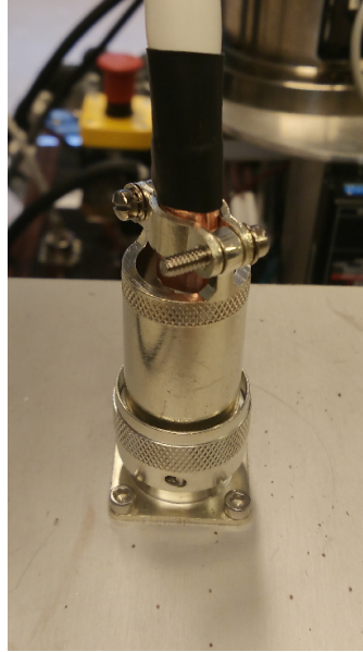
Figure 5.42: A burndy connector used for the test
