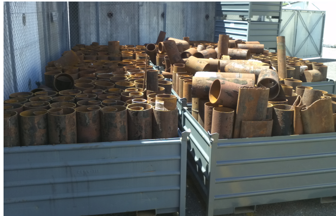
Figure 1.2: The PS pipes after the cutting process.
