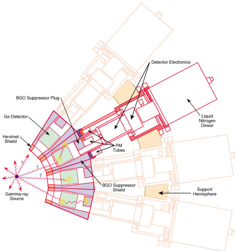
Figure 4.9.: Schematic transverse section of a Gammasphere HPGe detector, together with the BGO anti-Compton shield and the liquid nitrogen dewar. Image taken from [64].
