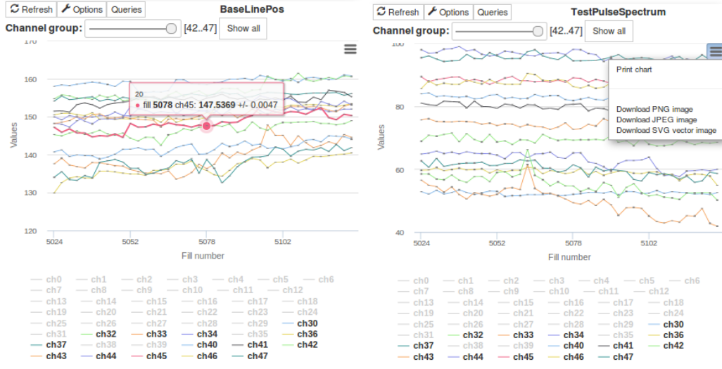
Figure 3.27: Left: The baseline positions for the set of channels as a function of the fill number. Right: The test pulse amplitude spectra mean value positions for the set of channels as a function of the fill number.
