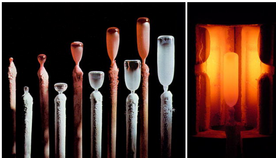
Figure 5.1: These photos show flame-fusion synthetic sapphire crystals, as-grown (left) and during growth in the furnace (right). Courtesy of Hrand Djevahirdjian, SA [101].
