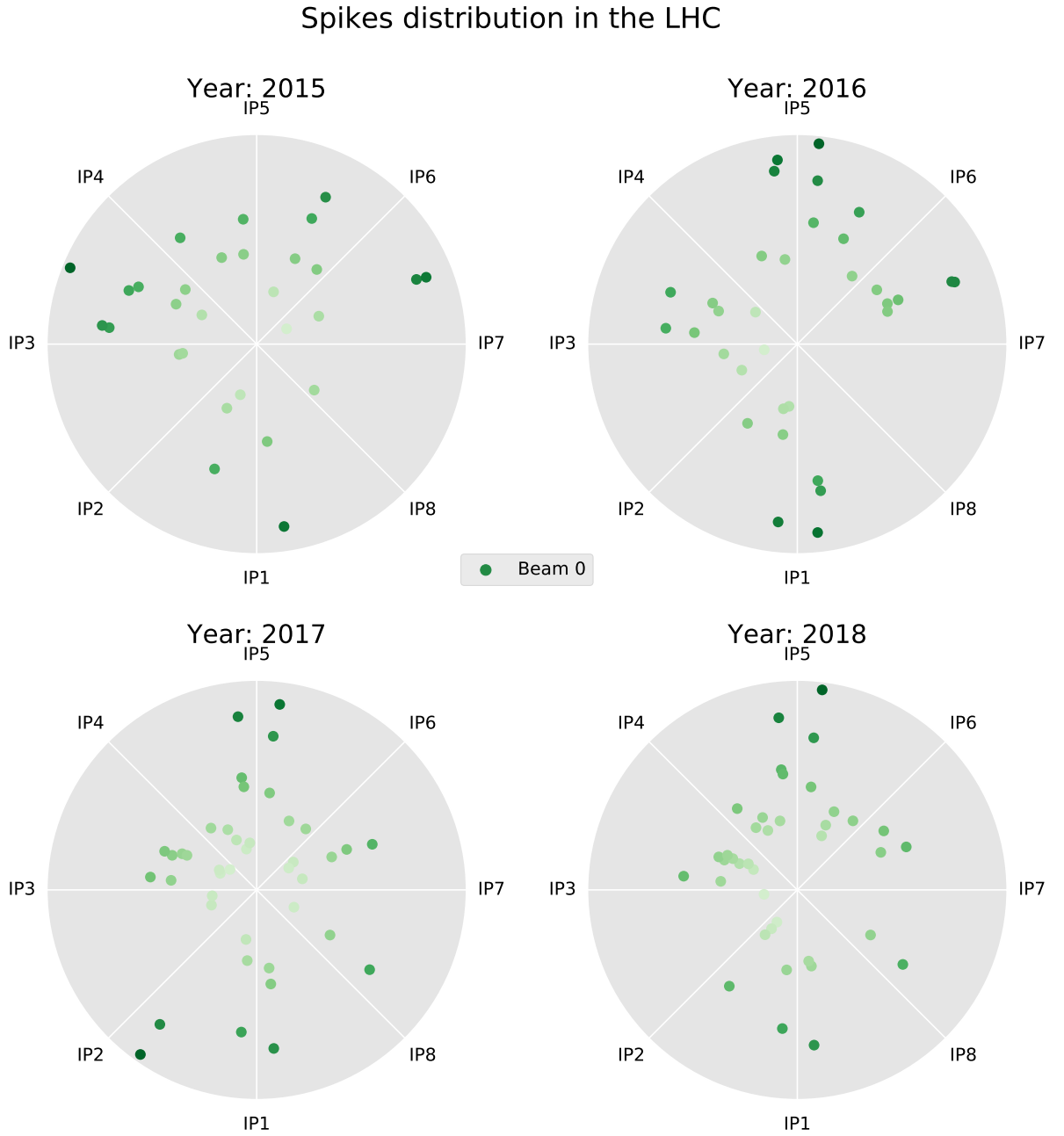
Figure 60: Spikes distribution in the LHC for different years. The radius and colour at the plot reflects the spike strength with respect to the highest spike in the top BLMs at the given year.
