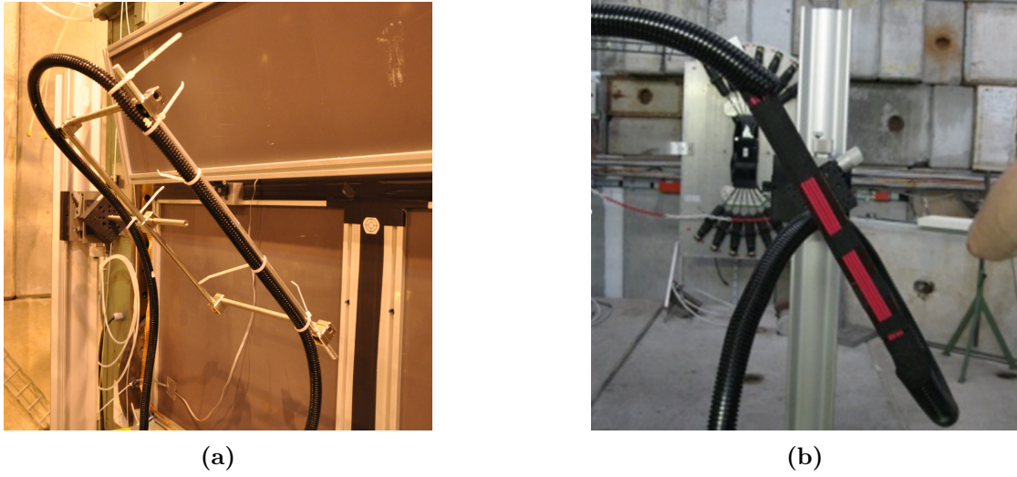
Figure 6.10: (a) The support used for the beam test in the CERN North Area in October 2011. The black tube containing the fiber was mounted on rotatable support. The beam was incident from the right. The scintillator used as a trigger is hidden in the box on the right side of the picture. (b) The fiber support used for the beam test in the CERN East Area in April 2012. The four fibers with different diameters (red) were placed behind each other, w.r.t. the beam direction. The beam is incident from the right.
