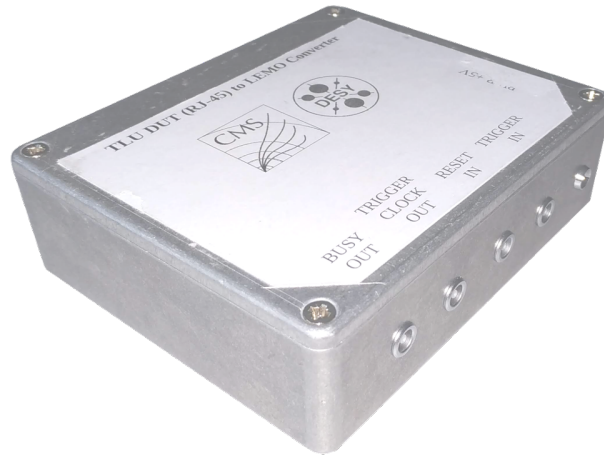
Figure A.2.: TLU RJ-45 to LEMO Converter.
