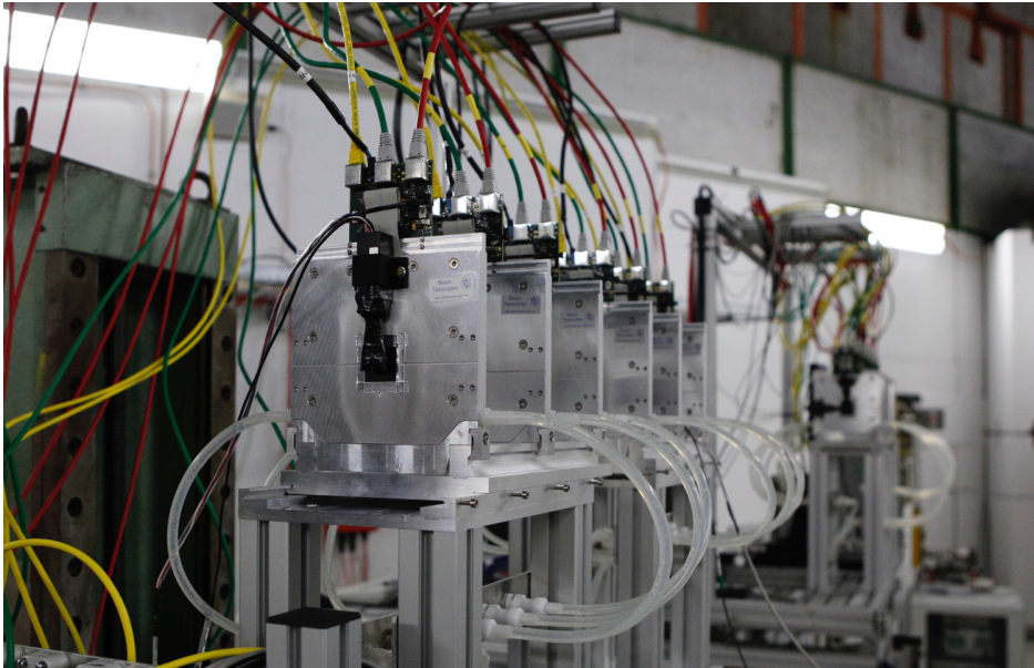
Figure 4.5.: EUDET-type telescopes at DESY [91].
