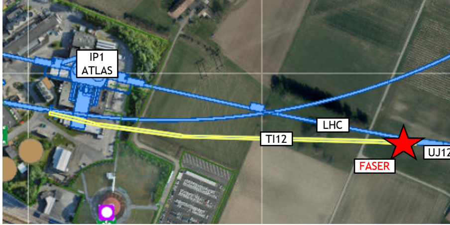
Figure 10.1: The location of the FASER detector at the LHC. The detector is located in the unused TI12 service tunnel 480 m from the ATLAS interaction point (IP1) along the beam collision axis line-of-sight with the LHC machine, concrete and rock in between. (Reproduced from Ref. [6], licensed under CC BY 4.0)
