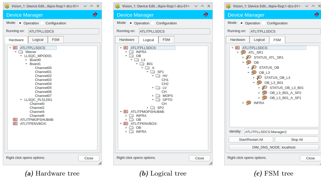
Figure 9.4: The Device Editor and Navigator showing the three different trees of the project. The hardware tree in (a) displays DP names, the logical tree in (b) displays alias names. Single operation panels can be opened from the hardware and logical view. The FSM follows closely the names of the logical tree. It can be started from the FSM view as shown in (c) and the corresponding GUI can be opened from there.
