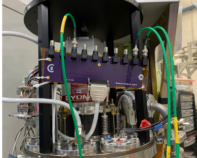
Figure 9.14: The room-temperature biasing breakout board is shown.
