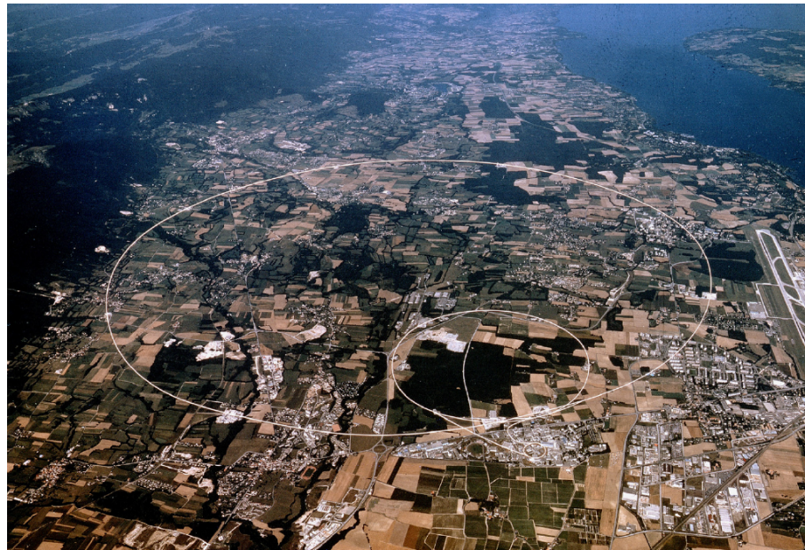
Figure 1: Aerial view of CERN and the surrounding region (CERN photograph, reprinted with permission). The 3 rings show the underground position of the accelerators. The smaller one is the Proton Synchrotron (PS), the middle ring is the Super Proton Synchrotron (SPS) with a circumference of 7 km and the largest ring (27 km) is the tunnel which housed the Large Electron Positron collider (LEP) and which will also house the Large Hadron Collider (LHC). Part of the Lake Geneva is visible in the background.
