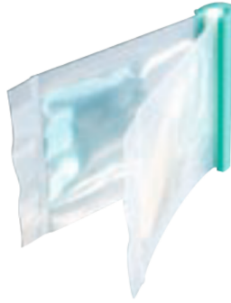
(a) Example of the pre-proportioned bags of Epolite FH-5313. The user removes the green plastic spacer and mixes the two component epoxy inside the bag.
