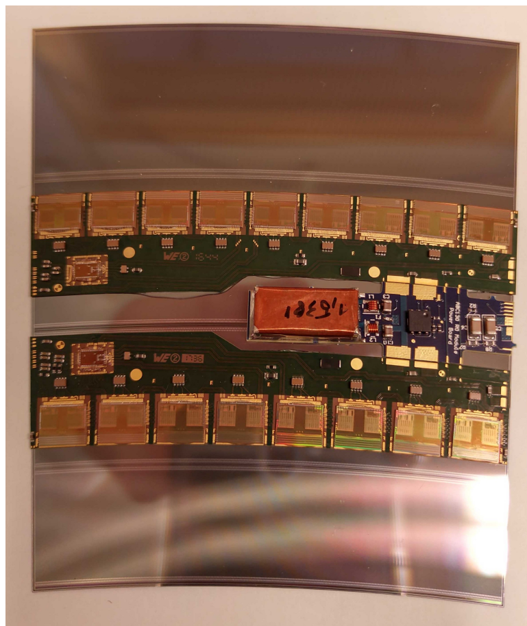
Figure 4.7: Top side view of the electrical R0, including the powerboard, prior to being shipped to Oslo for front-end wirebonding. The strips are going in the vertical direction. The segmentation of the four sets of strips can be seen by the lighter grey bands running horizontally across the sensor - with each hybrid being wirebonded to two of the segments.
