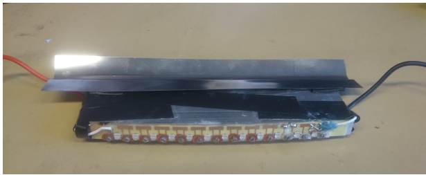
(c) LED bar, which attaches to the vacuum chuck and is used to cure the ASIC-to-hybrid glue. Metal blinders are mounted to contain the UV light - protecting the glue in the nearby semi-transparent syringe tip from prematurely curing.
