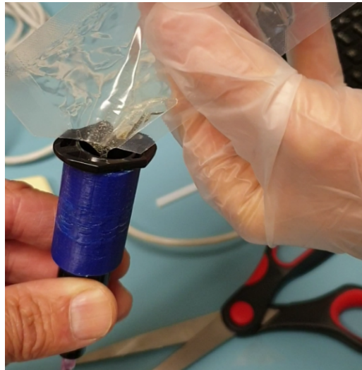
(b) Glue is poured in from the top of the syringe, then a plunger is added. Without the plunger the glue would just be pushed to the walls of the syringe instead of out through the needle.
