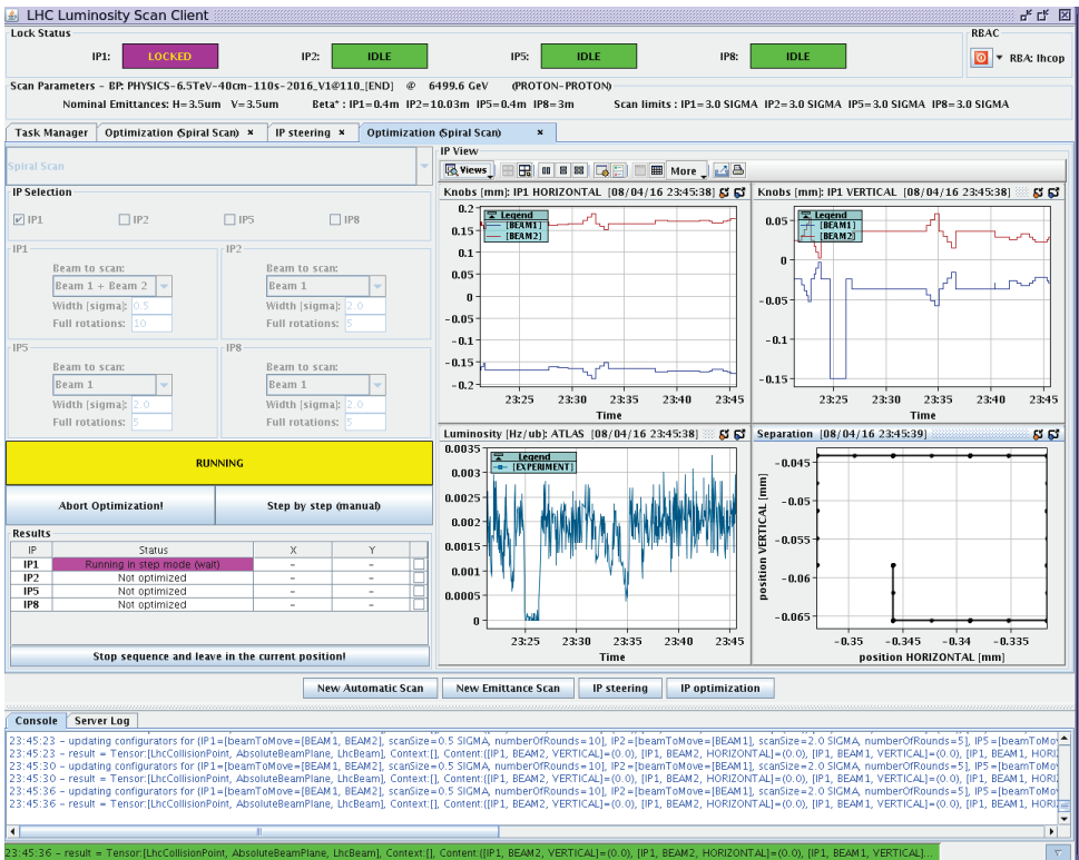
Figure C.6 – Finding collisions with a spiral scan (seen as a black line in the right bottom part, here in "rectangular form") on April 8 th 2016 when establishing first collisions after the winter stop in 2015/2016.
