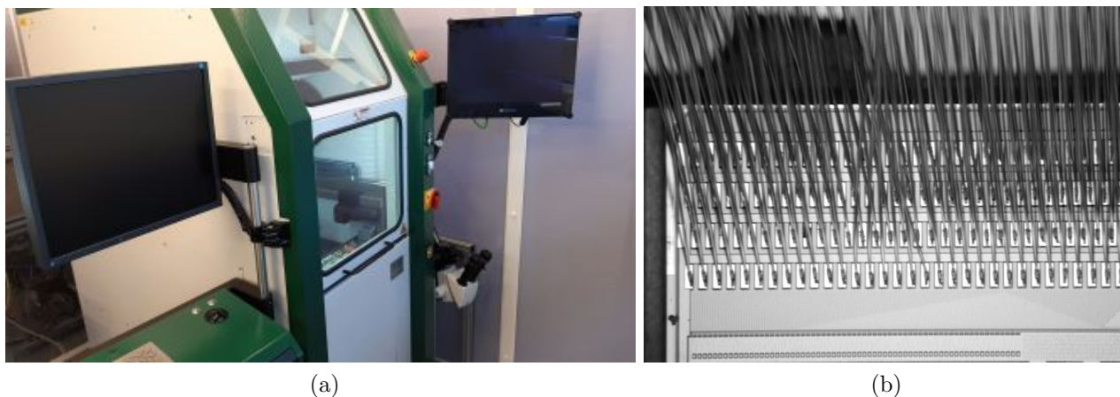
Figure 8.9: (a) The Hesse Bondjet BJ820 wire-bonder situated in the University of Sheffield clean room. (b) Sensor to ASIC wire-bonds shown for the module assembled in this section.
