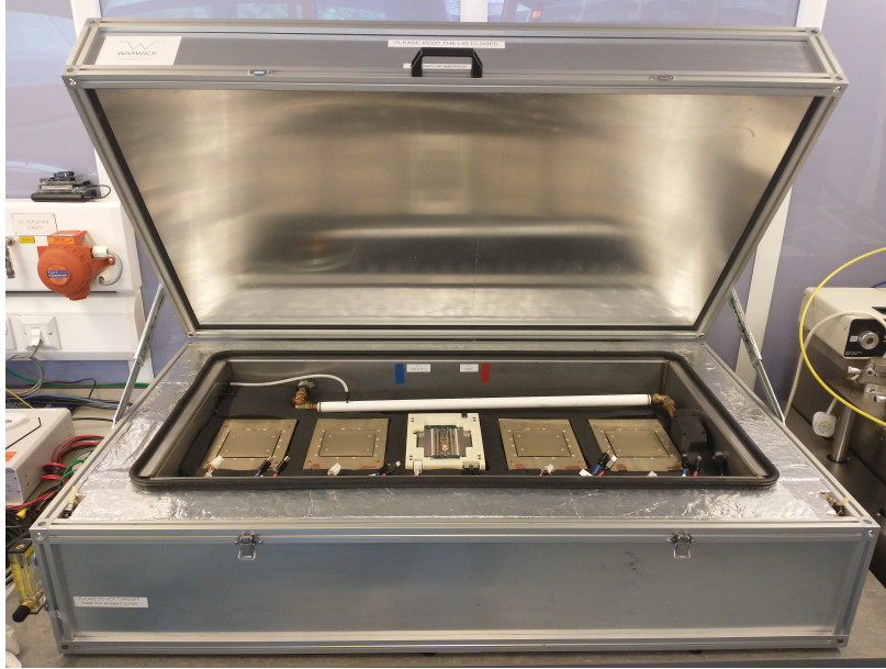
Figure 8.22: A photograph of the cold jig setup showing the five jigs and piping used for module thermal cycling. One completed module is placed in the centre jig ready for thermal cycling.
