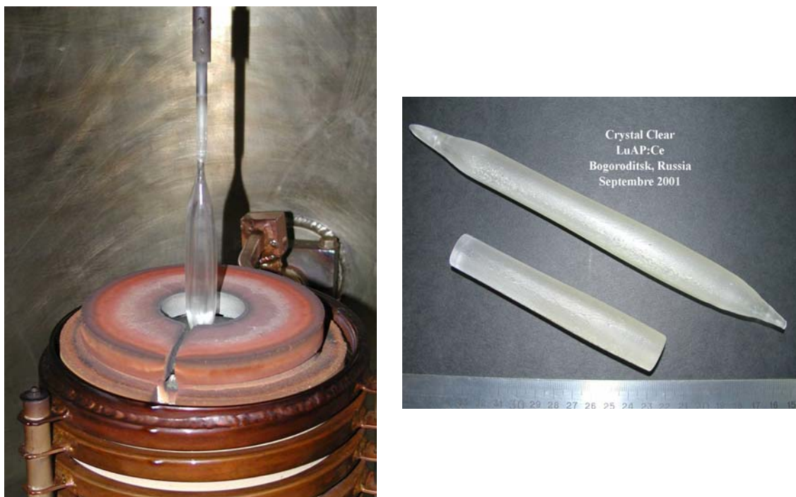
Figure 3.2 Pictures of the oven (left side) and of LuYAP ingots (right side) grown in the Bogoroditsk Techno Chemical Plant (Russia) in September 2001.
