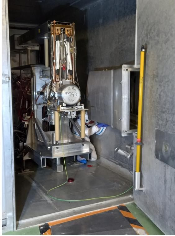
Figure 3.6 Picture of the HRS Faraday cage with the cover for MEDICIS target irradiations..
