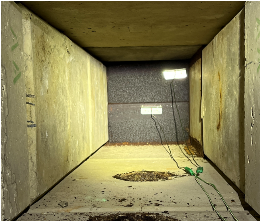
Figure 3.9 HRS dump face with both thermocouples installed..
