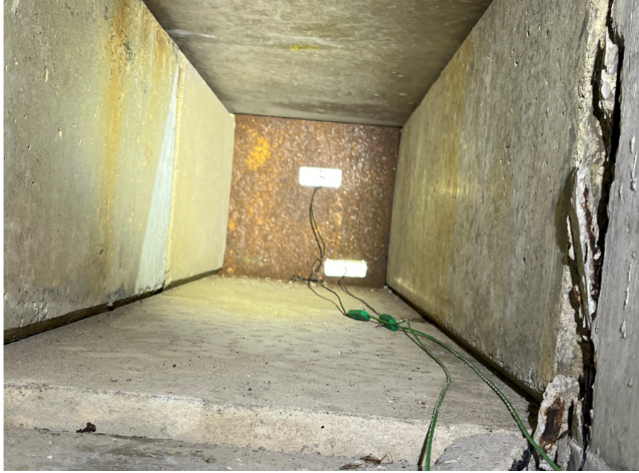
Figure 3.8 GPS dump face with both thermocouples installed..
