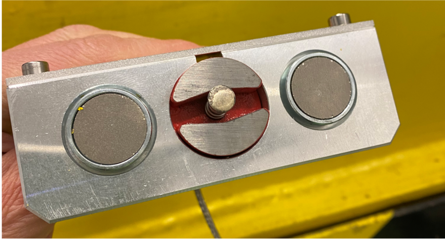
Figure 3.7 Thermocouple (center) with two magnets at each side. The thermocouple itself also includes magnets above and below..
