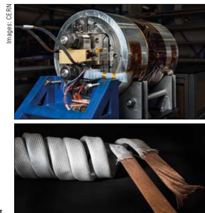
Top: The RMC_03 racetrack test magnet. Above: Samples of the two cables used to wind the RMC_03 coils.
