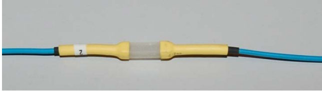
Figure 4.2 PMMA coated FBG packaging for pigtails protection
