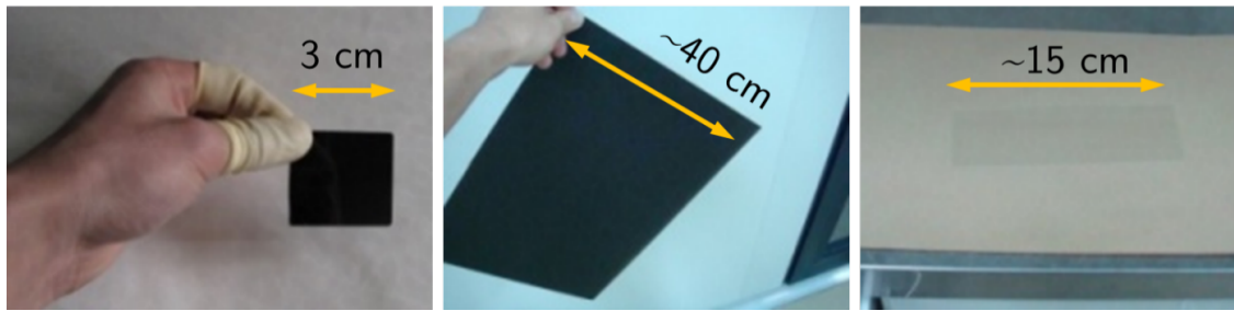
Figure 4.43 Photos of resistive materials. From left to right: semi-conductive glass, carbon-filled polycarbonate and regular floating glass.
