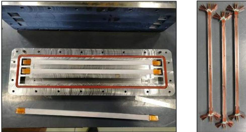
Fig. 3.8 - Impregnation mold used for the 4 cables stack impregnation study and a batch of impregnated 4 cables stack.
