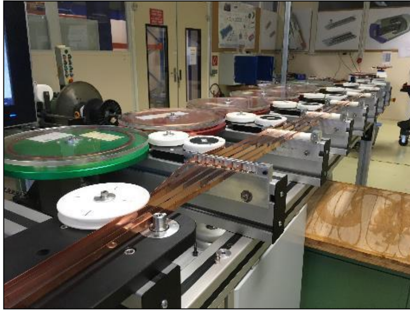
Fig. 3.6 - View of the multi-spool winding table assembled in the TE-MS-MDT laboratory.
