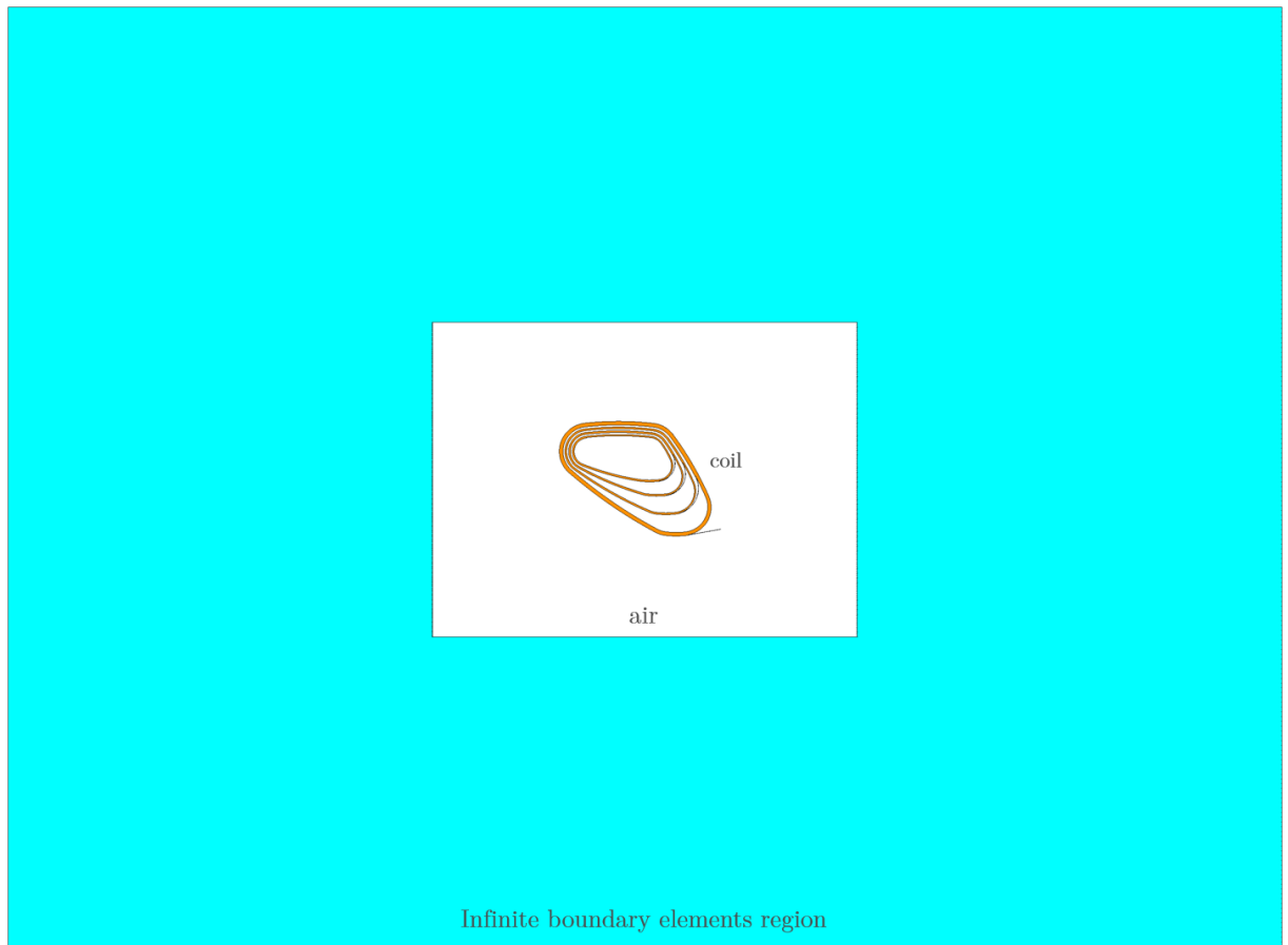
Fig. 5.3 – Schematic of the finite element model for electromagnetic calculations.
