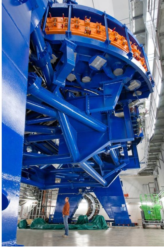
Fig. 2.5 – Picture of the HIT rotating gantry [15].
