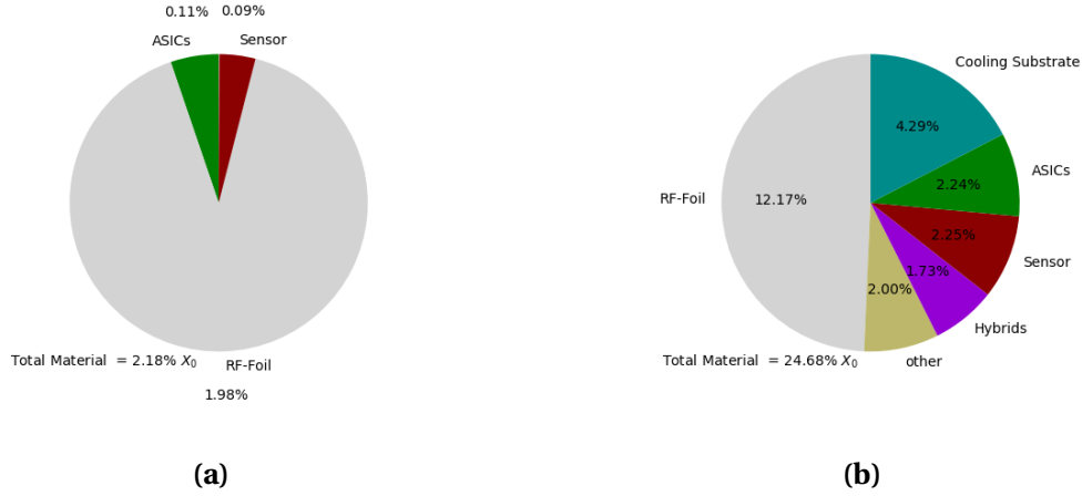
Fig. 4.8. Encountered material for the different components of the Upgrade I VELO up to the first measured point (a) and up to z = 82.5 cm (b).
