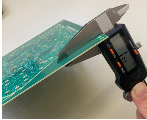
Figure 3.21: A practical demonstration of measuring the thickness of a board with a Vernier Caliper.
