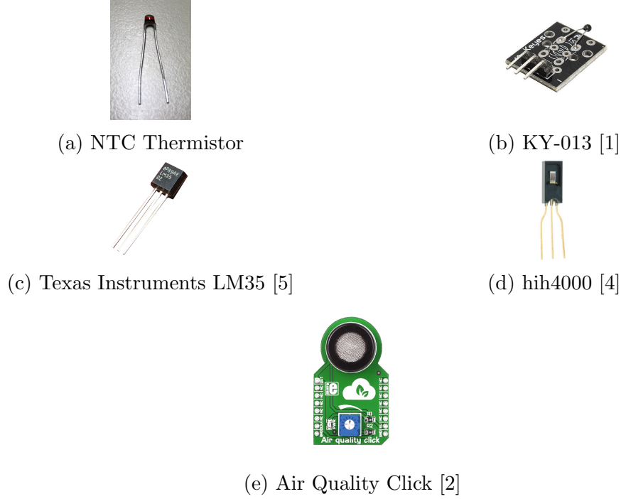
Figure 2: Sensors which used in the project
