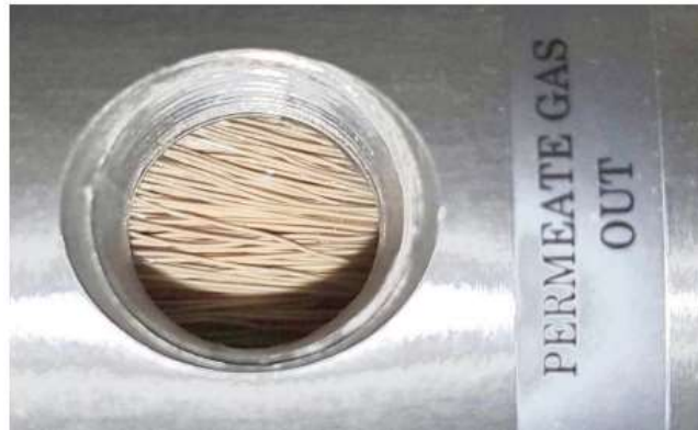
FIGURE 42: Picture of the UBE membrane section, with the bundle of straws visible inside the membrane case
