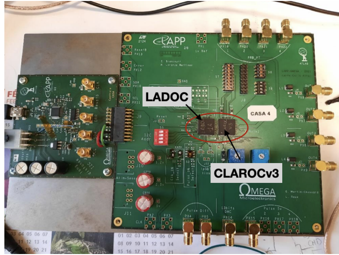
Figure 5.5.: Image of CASA test board, denoting its two main components: CLAROCv3 and LADOC
