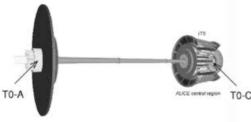
Figure 4.8: Position of the T0 detector inside ALICE detector setup [166].
