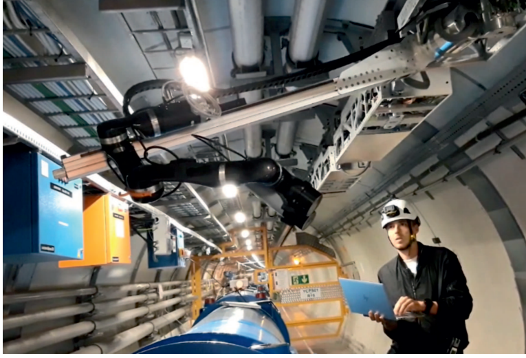
Figure 5.2: The Train Inspection Monorail (TIM) during testing in the LHC tunnel.
