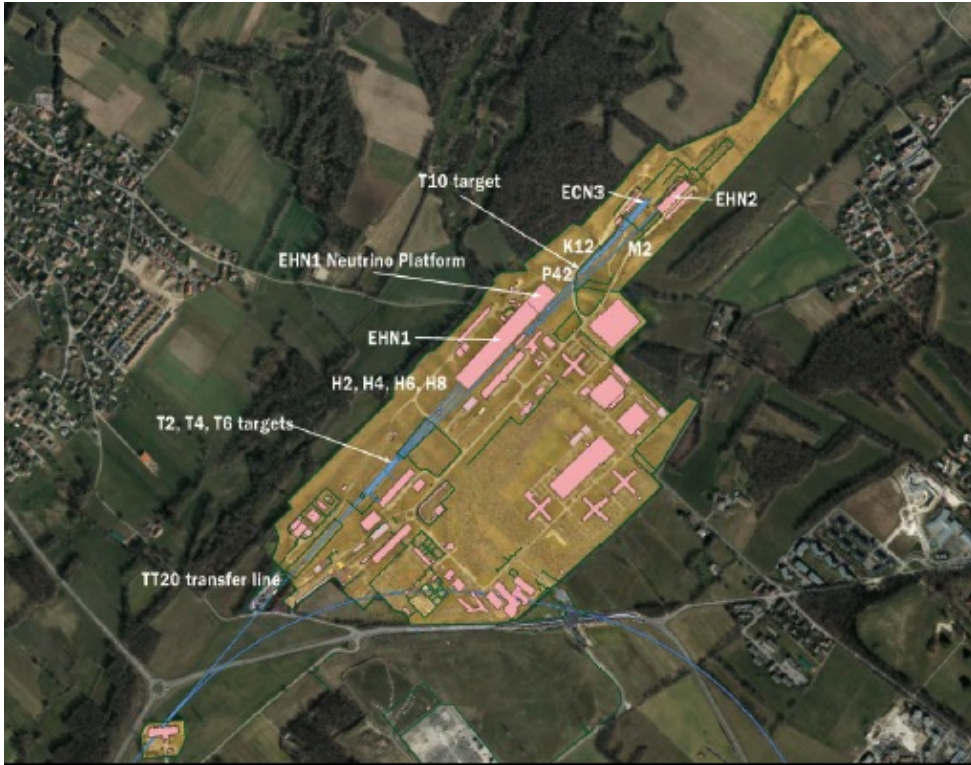
Figure 6.24: Aerial view of the CERN SPS north area, showing the layout of the halls, primary targets, and beam lines. The transfer lines transfer the primary beam to the primary targets. Image from [157].
