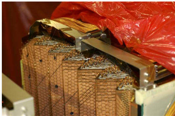
Figure 3.12: Accordion shaped calorimeter. Image from [78], © 2003-2024 CERN.
