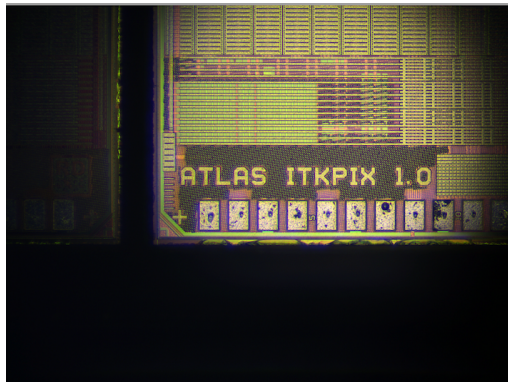
(d) Poor dicing and contaminated pad on Q10.
