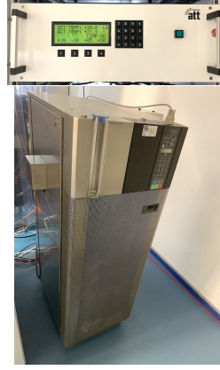
(b) Chiller and controller: Huber Unistat 380.
