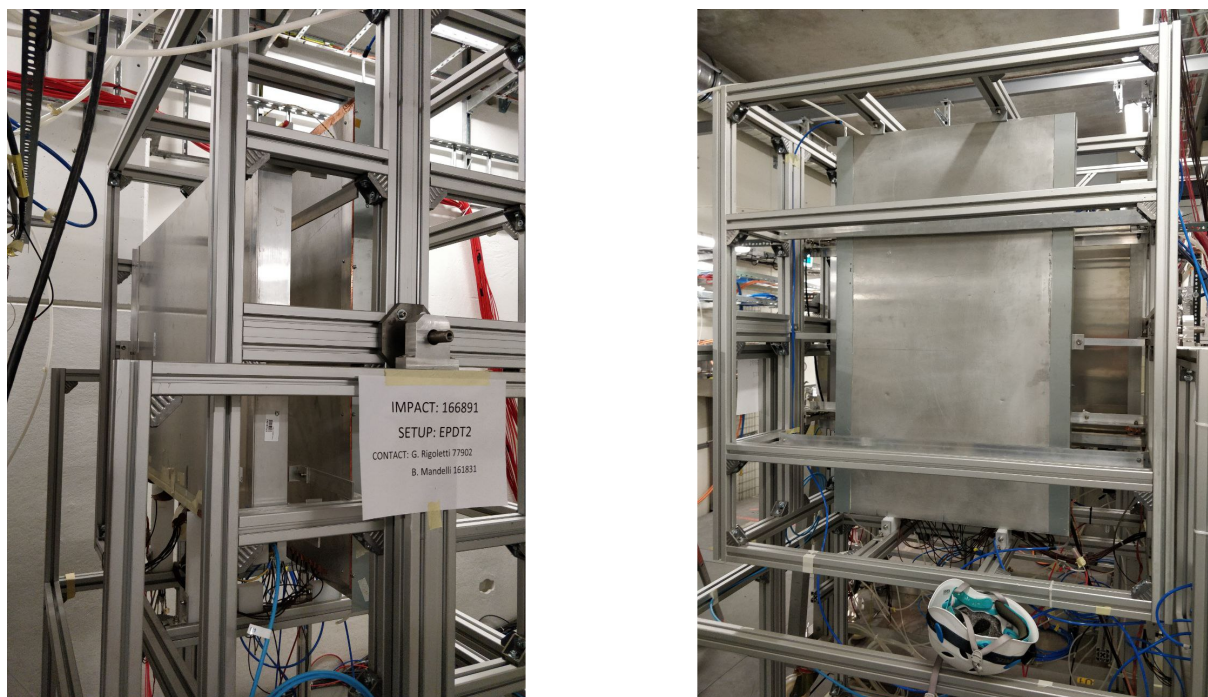
Figure 5.5: Metal structure for RPC installation inside the bunker trolley .
