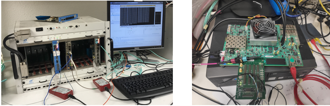
Figure 7.10: Test stands devoted to firmware-emulator comparison tests based on a Xilinx Virtex 7 FPGA (left), used with the previous AM algorithm version, and on a Xilinx Virtex Ultrascale Plus FPGA (right), used in the most recent tests.
