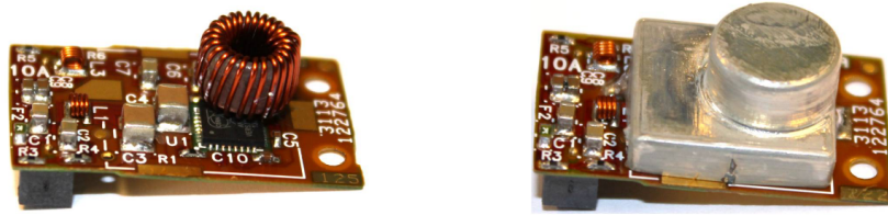
Figure 3.16: Photographs of a PIXV10 DC-DC converter, without (left) and with (right) the shield attached [35].
