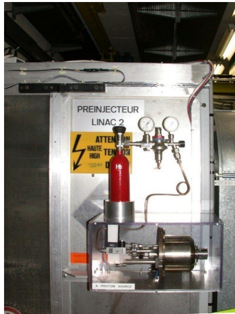
Figure 1.2: The hydrogen bottle that supplies protons to the LHC accelerator complex. [4]
