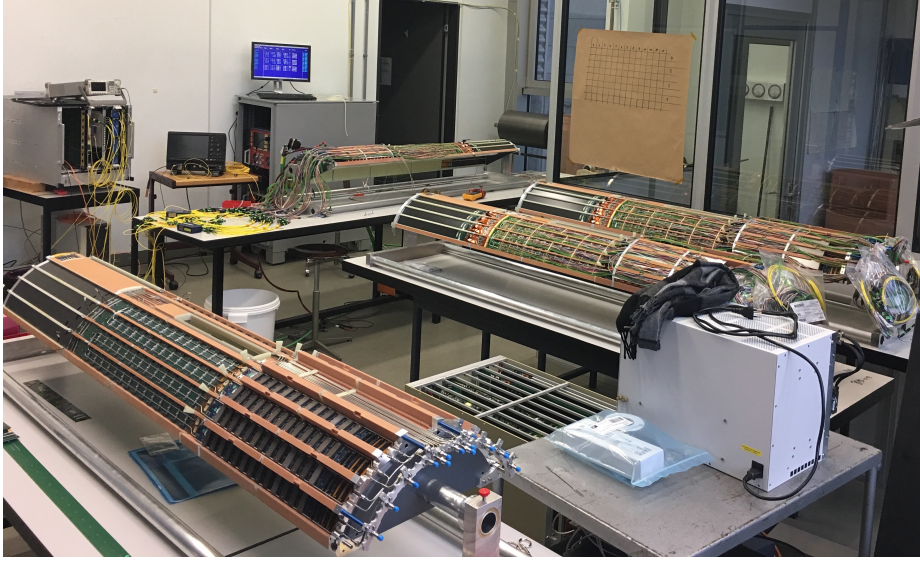
Figure 3.24: The four supply tubes in the UZH assembly room. The two on the right are already assembled and tested. The one on the bottom left corner is partially assembled and the cooling pipes and manifold are visible. The supply tube in the back is fully assembled and under test, the yellow optical fibres used to connect the supply tube to the DAQ system are visible on the table.
