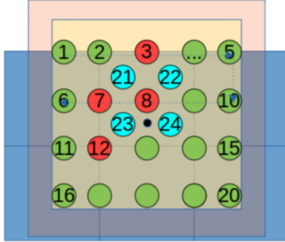
Figure 4.13: The different scan point positions used in the test beam. Scan point 8 represents the centre of the top middle ECAL module.
