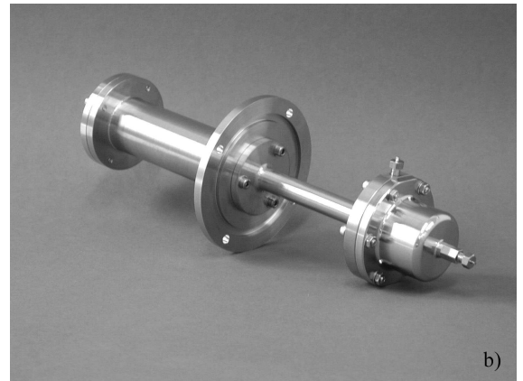
Figure 3.3: Images of the Cryogenic Micropump a) Rotor Image [33]; b) Prototype
