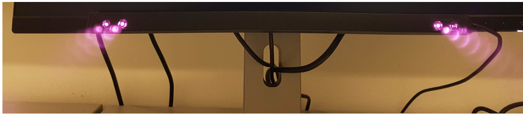
FIGURE 4.4: An example of a video-based eye tracker. The eye tracker is mounted below a computer screen. The model shown here is used in the studies presented in this thesis (cf. Section 5.2). The image was taken with a camera sensitive in the near-infrared range, which is why the near-infrared light emitted by the eye tracker is visible.
