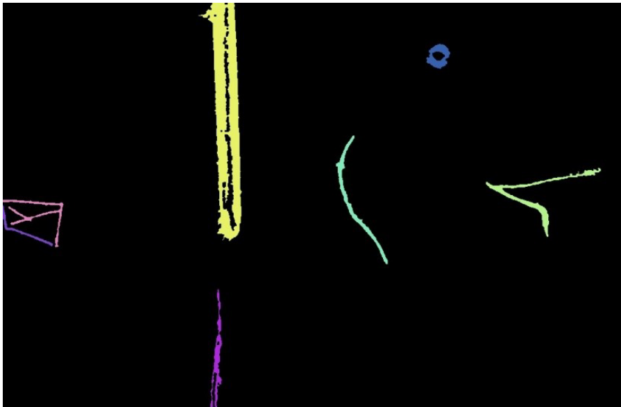
Figure F.22: Connected components labelling whereby neighbouring pixels are grouped and labelled as separate objects.
