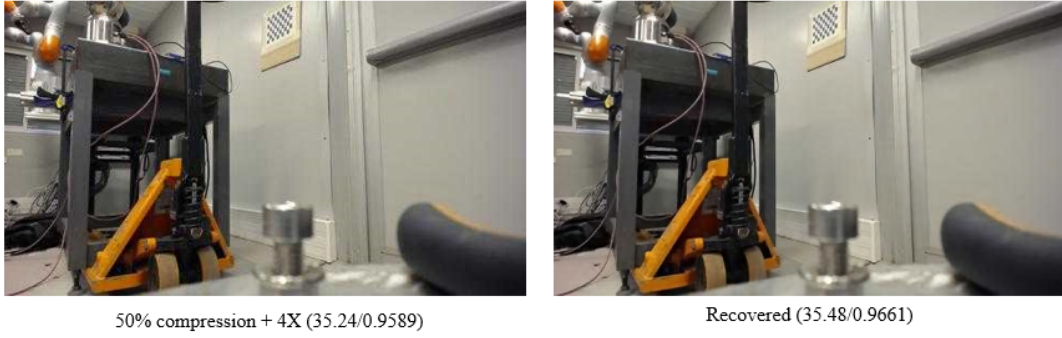
Figure 5.14: The 4X down-sampled image with 50% JPEG compression and the recovered image via DnCNN and ESPCN. The numbers in parentheses represent the peak signal-to-noise ratio (PSNR) and the structural similarity (SSIM), respectively.
