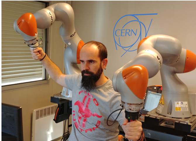
Figure C.2: Operator performing an intervention by the Master-Slave system with dual arms.
