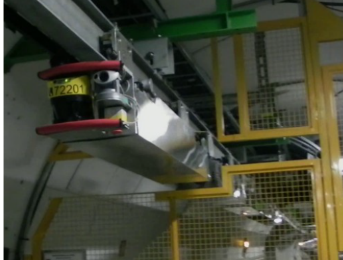
Figure F.3: TIM passing through sector doors passageways.
