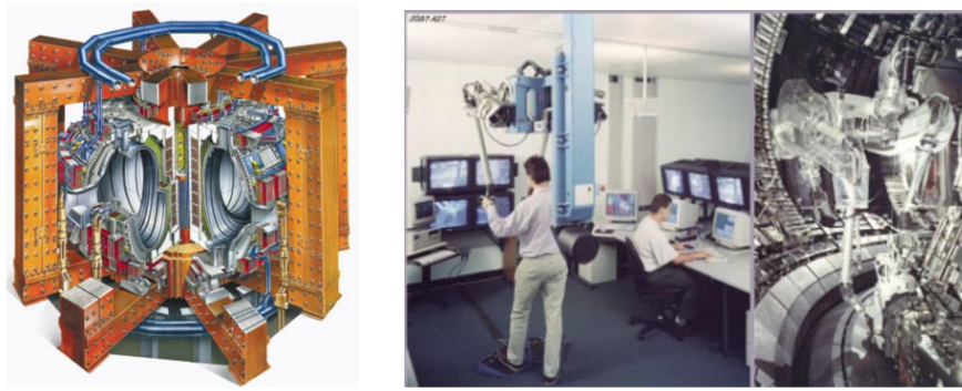
Figure 2.2: JET Torus (left) and remote handling approach using the MASCOT system [80] (Credit: www.euro-fusion.org )
