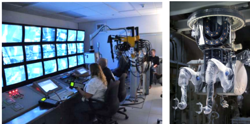
Figure 2.3: Remote handling control room (left) and the Telerob EMSM 2B telemanipulator system in use at SNS (Credit: www.ornl.gov )
