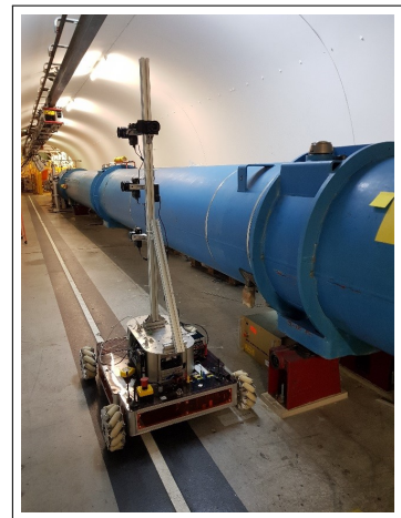
(b) CERNbot in tunnel mock-up
